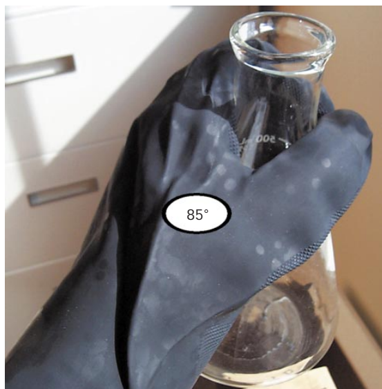
8 Industrial glove with hands-free thermometer (mock-up).
