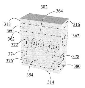
**Ex. 1001** at Fig. 3d; *see also*, *id.* at 9:24-27 ("As shown in FIG. 3d, the pressure sensor pad 354 may be configured in software to represent one or more delineated active areas corresponding to different programmable functions depending on the application."). The '692 Patent also describes two applications, a text application
