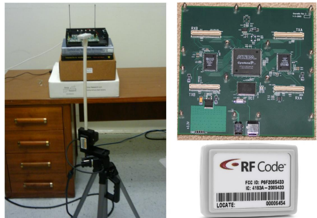
Fig. 1. The system setup (consisting a software-defined radio (USRP), RFID tags, and a pan-tilt unit) we have used for accurate manipulation and placement of tags for controlled experiments.
