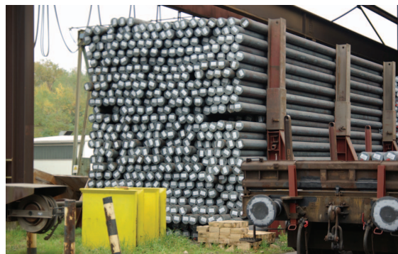
Figure 3. A cradle of steel billets implies only vague positional information. By individually tracking the billets' locations search times can be cut and optimized storing strategies can be implemented. Metal objects pose additional challenges to UHF RFID systems.
