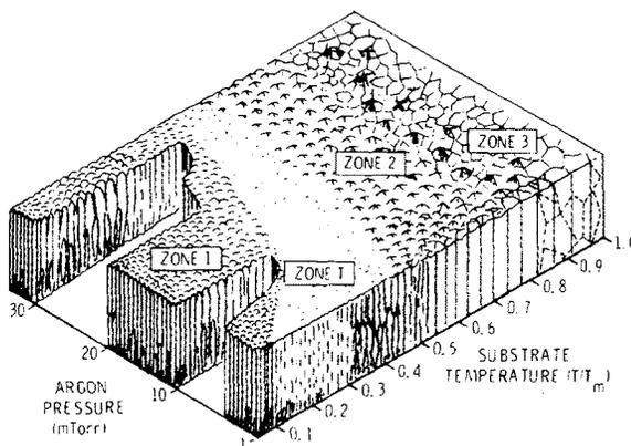
Fig. 1. Schematic representation of the influence of substrate temperature and argon pressure on the microstructure of metal coatings deposited using cylindrical magnetron sputtering sources.  $T$  (K) is the substrate temperature and  $T_m$  (K) is the melting point of the coating material. (See ref. 7.)
