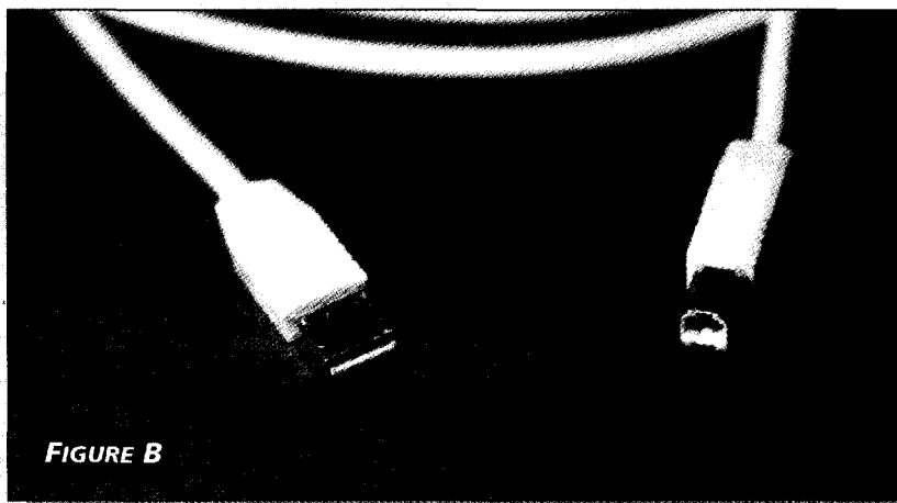
FIGURE B USB cable connectors come in two flavors. The flat connector is for devices with built-in cables. The second connector type allows detachable cables without the risk of cabling mistakes.
