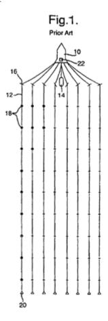
Figure 1, reproduced above, depicts an array of seismic streamers 12 towed behind the vessel. The '520 patent explains that in order to obtain accurate survey data, it is necessary to control the positioning of the streamers, both vertically in the water column, as well as horizontally against ocean currents and forces, which can cause the normally linear streamers to bend and undulate and, in some cases, become entangled with one another. *Id.* at col. 1, 1. 42–col. 2, 1. 25.
