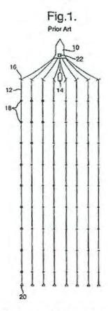
Figure 1, reproduced above, depicts an array of seismic streamers 12 towed behind the vessel. The '520 patent explains that in order to obtain accurate survey data, it is necessary to control the positioning of the streamers, both vertically in the water column, as well as horizontally against ocean currents and forces, which can cause the normally linear streamers to bend and undulate and, in some cases, become entangled with one another. *Id.* at col. 1, 1. 42–col. 2, 1. 25.
