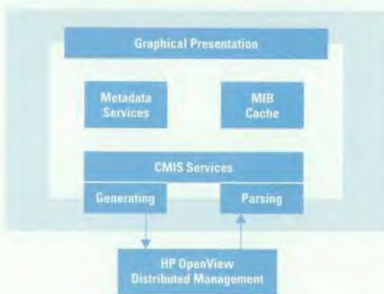
Fig. 8. The architectural framework for the three prototype tools.
