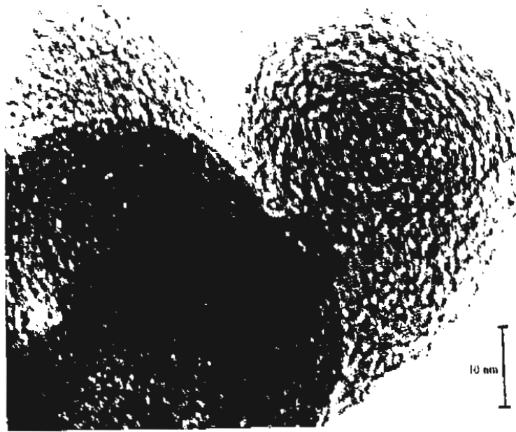
FIGURE 11-40 Lattice-imaging micrograph of a diesel particulate. 72
