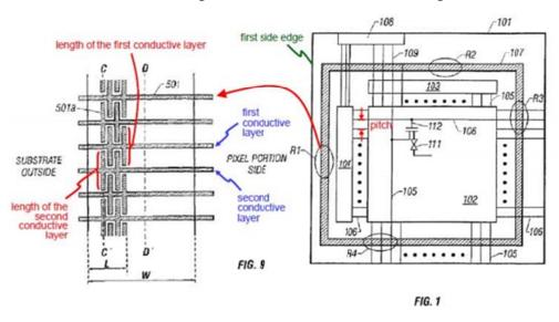
Figure 1 *supra* represents the top view of the lower substrate of an exemplary LCD device which incorporates, into the area R1 under seal 107, the dummy wiring structures depicted in adjacent Figure 9. (*See* Prelim. Resp. 14-16.)
