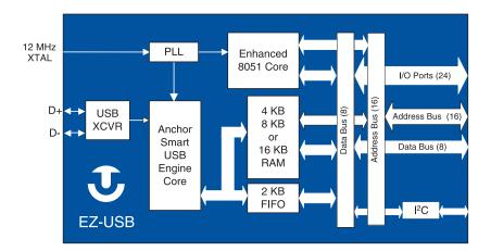
The Anchor Chips EZ-USB™ family (AN21XX/AN23XX) provides significant improvements over other USB architectures including an enhanced 8051 core, 4, 8 or 16 Kbytes of RAM, an intelligent USB core, and high-performance I/O ports. The family includes 16 different products to accommodate the needs of different systems.
