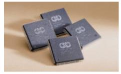
CMD's proprietary RAID chipset is the key to the CRD-5500's advanced features and incredible performance. Four separate ASICs for RAID (Exclusive OR), cache control, CPU-I/O (CPU support logic), and DMA (high speed internal data bus)
