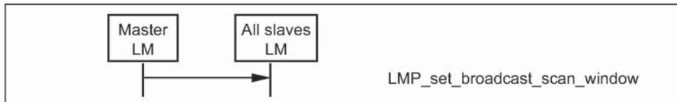
Sequence 38: Master notifies all slaves of increase in broadcast capacity.
