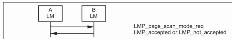
Sequence 58: Negotiation for page scan mode
