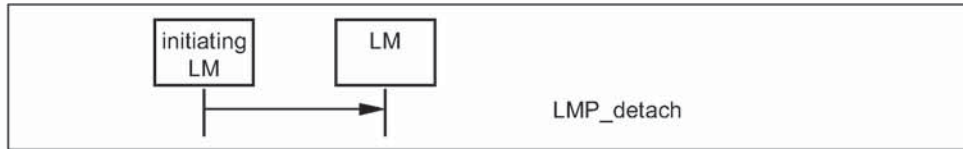
Sequence 26: Connection closed by sending LMP_detach.
