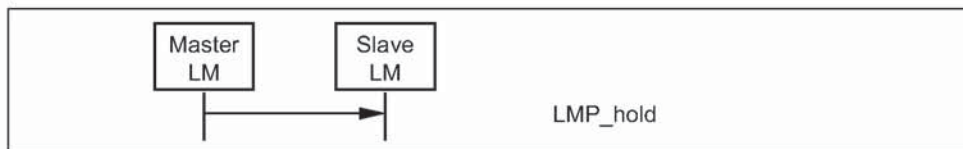
Sequence 27: Master forces slave into hold mode.
