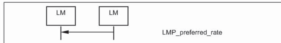
Sequence 46: The right-hand device orders the left-hand device to change data rate.
