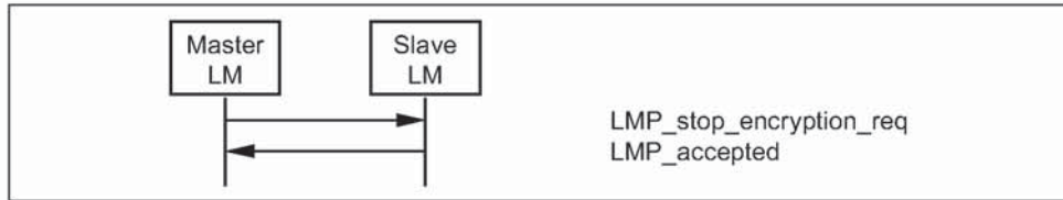
Sequence 16: Stop of encryption.
