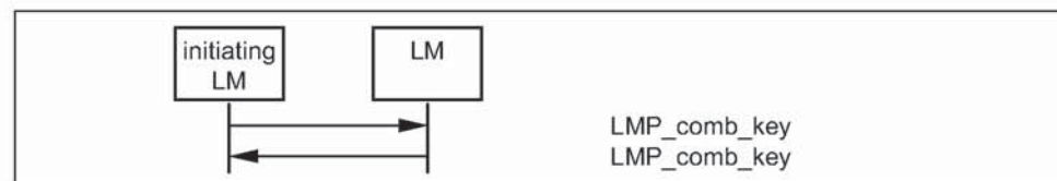
Sequence 8: Successful change of the link key.
