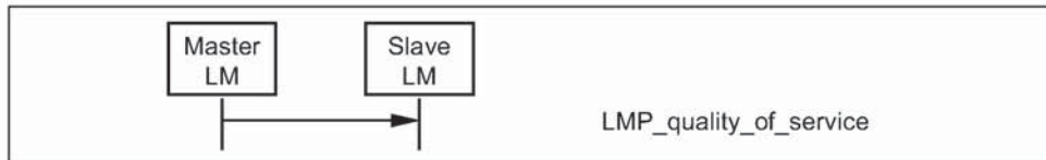
Sequence 47: Master notifies slave of new quality of service.
