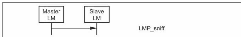
Sequence 30: Master forces slave into sniff mode.
