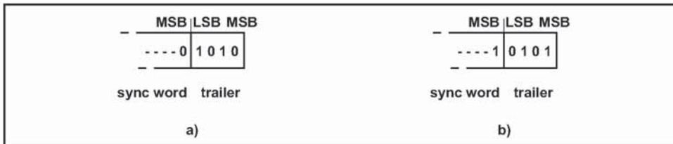
Figure 4.4: Trailer in CAC when MSB of sync word is 0 (a), and when MSB of sync word is 1 (b).
