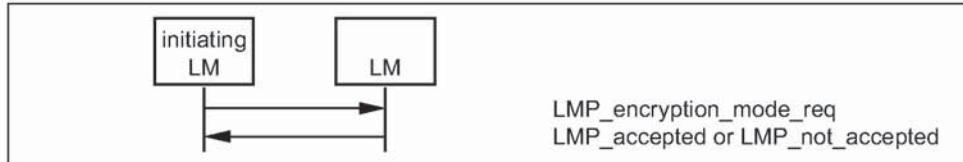
Sequence 12: Negotiation for encryption mode.
