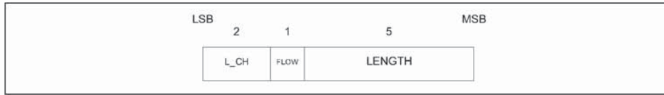
Figure 1.2: ACL Payload Header for single-slot packets
