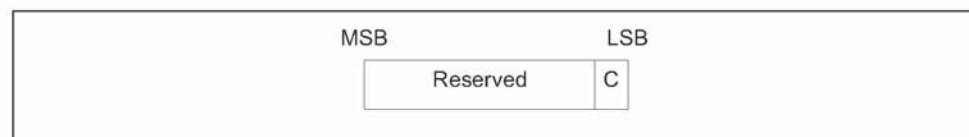
Figure 5.7: Configuration Request Flags field format
