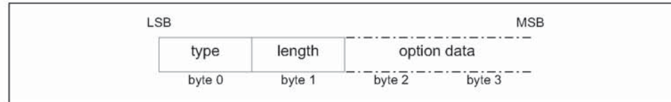
Figure 6.1: Configuration option format
