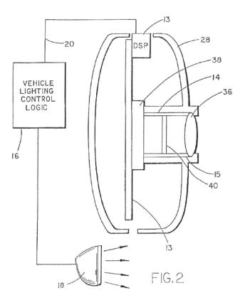
Figure 2 of the '552 patent is a partial side view of a vehicle headlight dimming control system.
