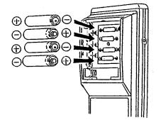
3. If you are installing batteries for the first time, press and hold [CANCEL]. Then, use a pen or pencil to press [RESET] inside the battery compartment. The reset feature is a two-key sequence to prevent accidental use.
