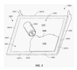
Figure 3 illustrates a preferred embodiment that includes shelving with a spill containment pattern consisting of a hydrophobic surface in the pattern of a frame-like border. *Id.* at col. 2, ll. 26-30; col. 3, ll. 43-45. The border defines the boundaries of a single non-hydrophobic spill containment area therein. *Id.* at col. 3, ll. 39-46.
