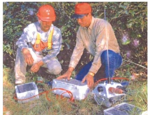
The VectorSeis System Four VR incorporates TrueDigital microelectromechanical systems accelerometers to image structural and stratigraphic detail in land and transition zone environments.
