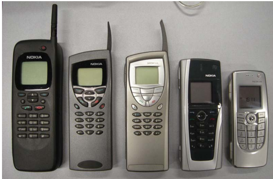
The diminishing size of Nokia Communicators from 1996 to 2004. From left: Nokia 9000, 9110i, 9210i, 9300 and 9500 / Sergio Oliveira
