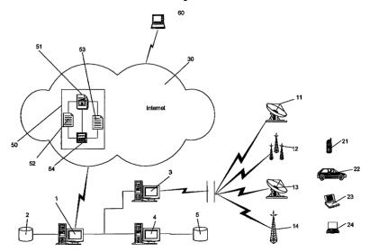
Figure 1 illustrates mobile platforms, including mobile telephone 21, car 22, laptop 23, and briefcase 24, and location tracking systems 11, 12, 13, 14 that communicate with communication subsystem 3 of location determination system 1. Ex. 1101, col. 3, ll. 31–32; col. 3, l. 44–col. 4, l. 11. Location determination system 1 is linked to database 2 and map server 4
