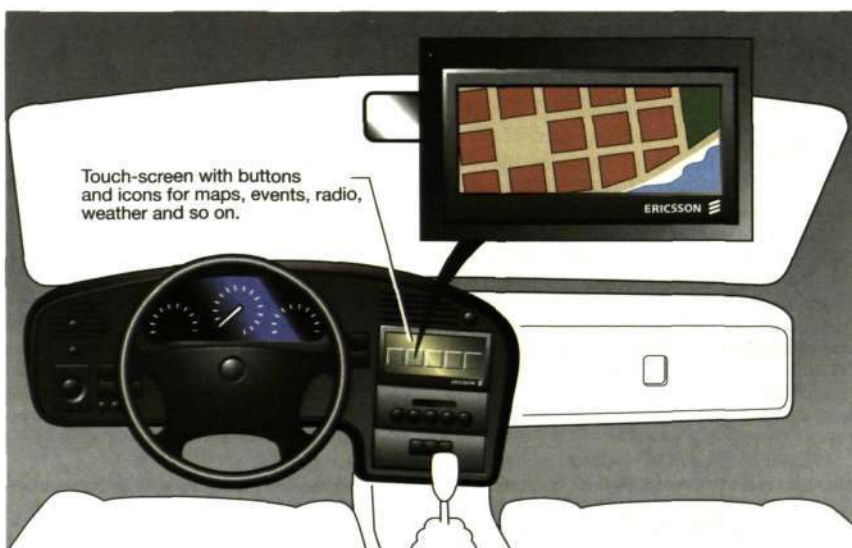
Figure 1 The user has easy access to online services via a touch-screen that is connected to a GPRS-enabled terminal. The touch of one icon brings up a map of the area; the touch of another icon calls up a report on current traffic conditions; the touch of still another icon fetches current events in the area (concerts, parades, and so on).
