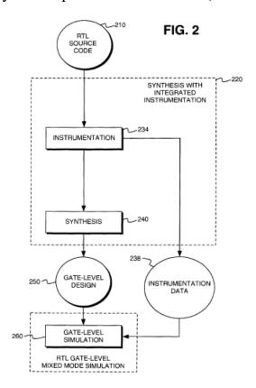
Figure 2, above, shows that RTL source code 210 is provided to synthesis process 220, which includes instrumentation step 234 followed by synthesis step 240. *Id.* at II. 11-16. In the first embodiment, in which the gate level netlist is modified to include instrumentation signals, the resulting gate-level design 250 "contains additional logic to create the additional instrumentation output signals referenced in instrumentation data 238." *Id.* at II. 17-30.
