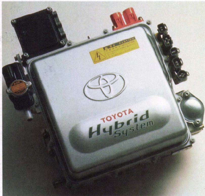
Prius' high-output nickel-hydride battery pack (top) is positioned between the rear seat and luggage compartment. Below is the inverter unit, whose electronic elements are of Toyota's own design and manufacture, as is the motor regenerator.
