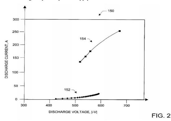
Figure 2 shows current-voltage characteristic 154 that represents actual data for plasma generated by the pulsed power supply in the plasma
