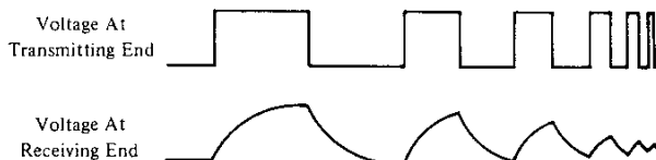
FIGURE 2.1 Attenuation of Digital Signals
