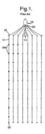
Figure 1 depicts an array of seismic streamers 12 towed behind the vessel.
