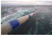
Towing deep in a quiet environment with collocated pressure and velocity sensors improves operational performance and efficiency.
