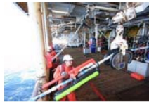
Towing deep in a quiet environment with collocated pressure and velocity sensors improves operational performance and efficiency.
