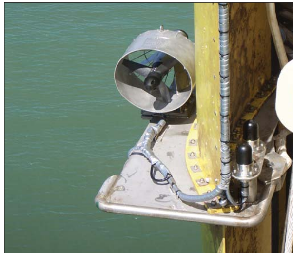
Figure 4: Baro48 paravane on a PGS Ramform vessel a generator and acoustic pingers mounted.
