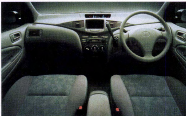
Instrumentation is digital, in the center top of the instrument panel, below which is a multipurpose display.
