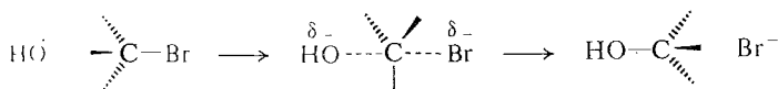
Figure 5.2 The S N 2 reaction: complete inversion of configuration. The nucleophilic reagent attacks the back side.
