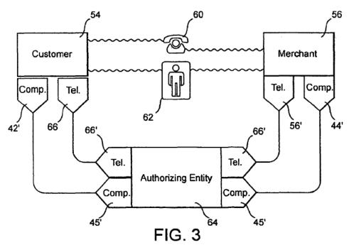
Figure 3 of the '988 patent is reproduced below:
