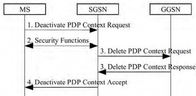
Figure 41: PDP Context Deactivation Initiated by MS Procedure
