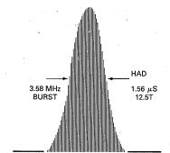
Envelope of frequency spectrum of modulated 12.5T pulse
