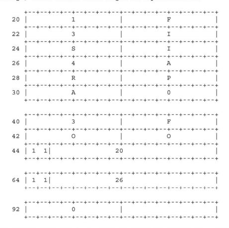
The domain name for F.ISI.ARPA is shown at offset 20. The domain name FOO.F.ISI.ARPA is shown at offset 40; this definition uses a pointer to concatenate a label for FOO to the previously defined F.ISI.ARPA. The domain name ARPA is defined at offset 64 using a pointer to the ARPA component of the name F.ISI.ARPA at 20; note that this pointer relies on ARPA being the last label in the string at 20. The root domain name is
