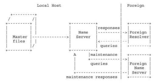
In this configuration, the name server periodically establishes a virtual circuit to a foreign name server to acquire a copy of a zone or to check that an existing copy has not changed. The messages sent for
