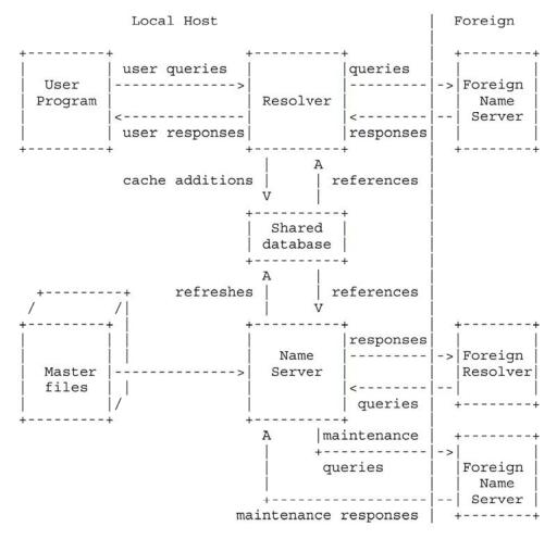
The shared database holds domain space data for the local name server and resolver. The contents of the shared database will typically be a mixture of authoritative data maintained by the periodic refresh operations of the name server and cached data from previous resolver requests. The structure of the domain data and the necessity for synchronization between name servers and resolvers imply the general characteristics of this database, but the actual format is up to the local implementor.
