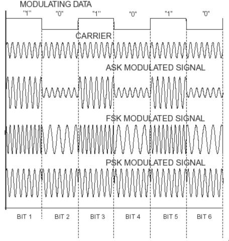
The top trace is the information signal, and the second trace is the carrier. The three remaining traces show what happens to a carrier when it is modulated with a digital data stream using ASK, FSK, and PSK modulation techniques. Several forms of pulse modulation are illustrated in the following figure.
