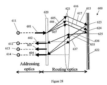
Figure 28 of the '710 patent illustrates wavelength routing and selection device 600.
