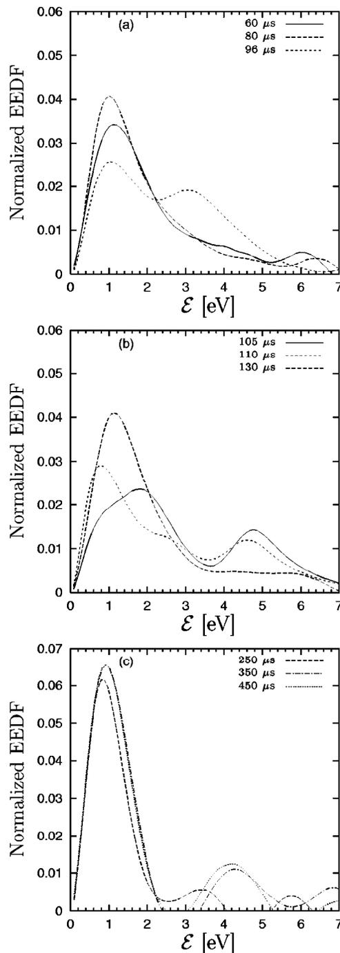
FIG. 1. Normalized EEDF measured (a) during pulses 60, 80, and 100  $\mu\text{s}$  after initiating the pulse; (b) around the electron density maximum 105, 110, and 130  $\mu\text{s}$  after initiating the pulse; and (c) 250, 350, and 450  $\mu\text{s}$  after initiating the pulse. Pulse length, 100  $\mu\text{s}$ ; average power, 300 W; and pressure 2 mTorr.
