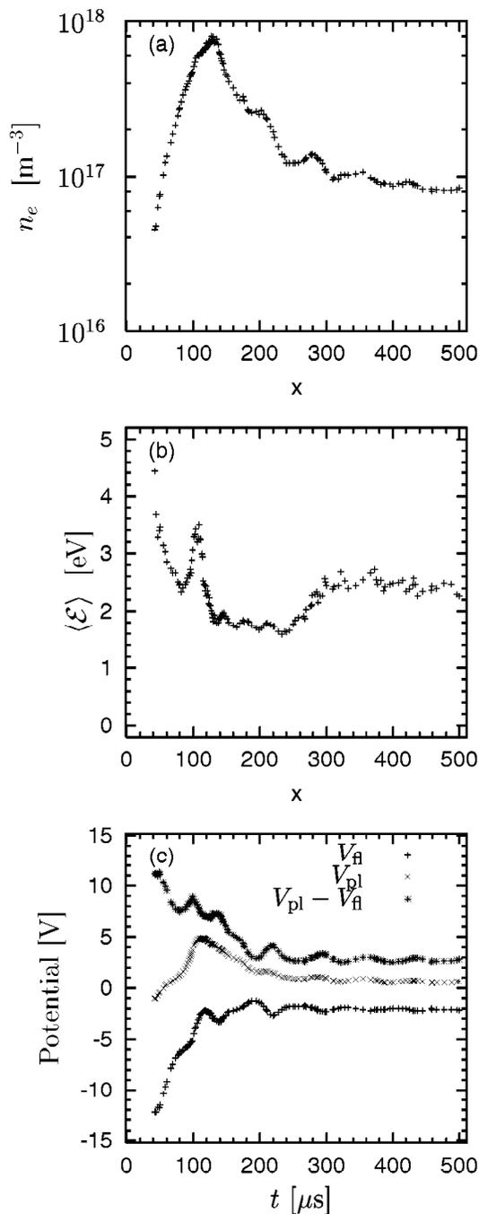
FIG. 2. (a) Electron density, (b) average electron energy, and (c) + floating potential  $V_{fl}$ ,  $\times$  plasma potential  $V_{pl}$ , and \* potential difference ( $V_{pl} - V_{fl}$ ) as a function of time from initiation of the pulse. Target current pulse length, 100  $\mu\text{s}$ ; average power, 300 W; and pressure, 2 mTorr.
