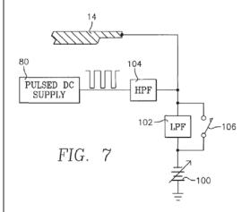
Wang at 7:61-62 ("The pulsed DC power supply 80 produces a train of negative voltage pulses.").
