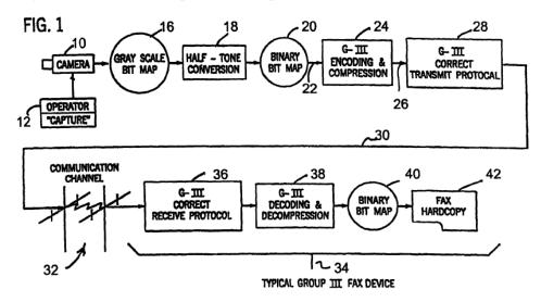
"Figure 1 is a block diagram of a basic facsimile camera configuration for capturing an image via a camera and transmitting it via Group III facsimile transmission to a standard hard copy medium." *Id.* at 4:27-30.
