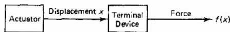
Figure P2.33. Block diagram for a terminal device of a robotic manipulator.
