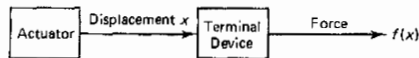
Figure P2.33. Block diagram for a terminal device of a robotic manipulator.
