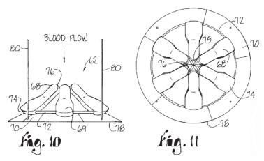
Figures 10 and 11 illustrate a diagrammatic and plan view of one embodiment of Dr. Norred's cone-shaped aortic valve in a closed position.
