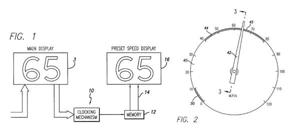
Figure 1 illustrates a digital speed display, while Figure 2 illustrates an analog speedometer. *See id.* at 3:8-13. In Figure 1, main speed display 3 shows the current speed at which the vehicle is operating. *See id.* at 3:49-53. When a cruise control set button (not shown in Figure 1) is pressed, the vehicle speed is stored in digital memory 12 as a preset speed. *See id.* at 3:53-60. Second speed display 16 shows that preset speed. *See id.*
