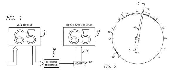
Figure 1 illustrates a digital speed display, while Figure 2 illustrates an analog speedometer. *Id.* at 3:8–13. In Figure 1, main speed display 3 shows the current speed at which the vehicle is operating. *Id.* at 3:49–53. When a cruise control set button (not shown in Figure 1) is pressed, the vehicle speed is stored in digital memory 12 as a preset speed. *Id.* at 3:53–60. Second speed display 16 shows that preset speed. *Id.*
