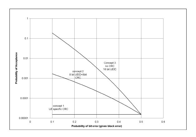
Figure 1 Probability of false acceptance versus conditional bit error probability for an erroneous block intended for the receiving UE
