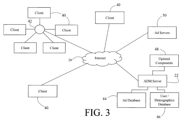
Figure 3 illustrates a block diagram of a system distributing advertisements over the Internet. *Id.* at col. 6, ll. 21–22. ADM server 22 is accessible by client computers 40 over Internet 20, where client computers 40 have the client software application installed. *Id.* at col. 8, ll. 32–35. ADM server has associated with it
