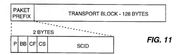
Menand discloses that the packet prefix includes a twelve-bit field for the SCID. (*Id.* at 6:51-53.) The program controller of Menand assigns "respective SCID's for respective audio, video and interactive components of respective programs." (*Id.* at 2:49-51.)
