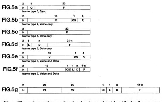
28. These frames have a header that is used to identify the frame type, as shown in the table below:
