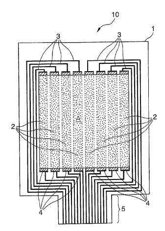
(57) Abstract: The present invention discloses a touch panel sensor comprising: (a) a transparent flexible substrate, (b) a transparent conductive film formed on the transparent flexible substrate, (c) wiring composed of a metal or metal alloy, and (d) electrodes composed of conductive ink or paste for connecting the transparent conductive film (b) and the wiring (c).
